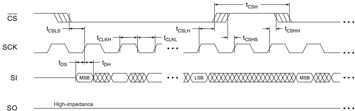
Figure 14-2. Serial Output Timing
