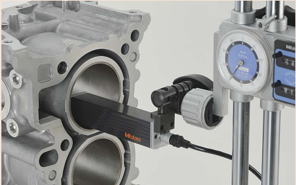
Can be combined with height gage for easy positioning.
