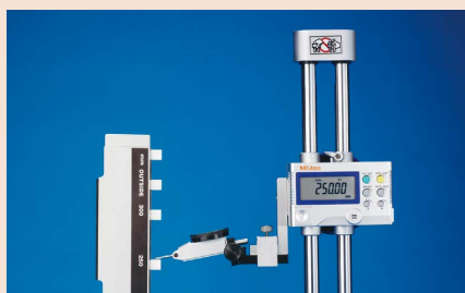
Checking accuracy of height gage
