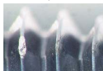
SC-TL-RZ After 7,000 holes
