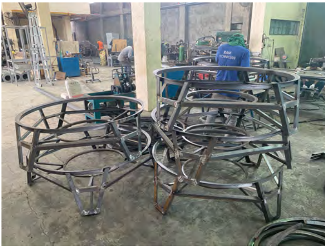
Stainless steel tank frames in our shop
