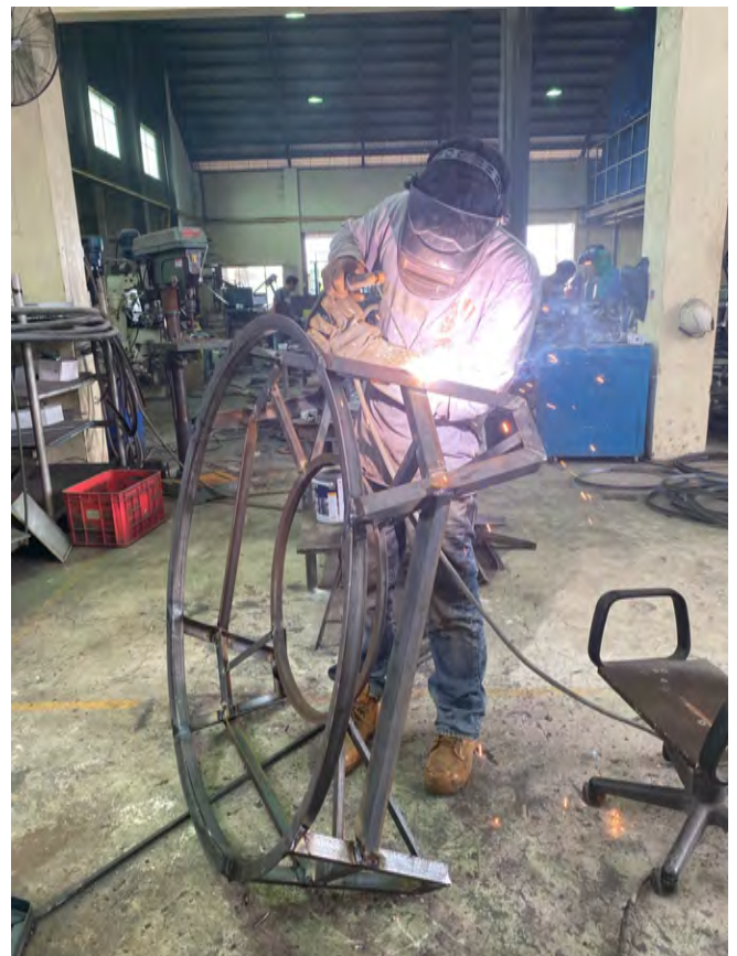
Manufacturing personnel working on stainless steel tank frames, part of AIDFI's income generation
