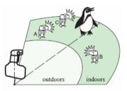
Press the test button of master to test whether the flash works normally; if the flash does not fire, adjust the slave unit's angle toward the master unit and distance from the master unit.
