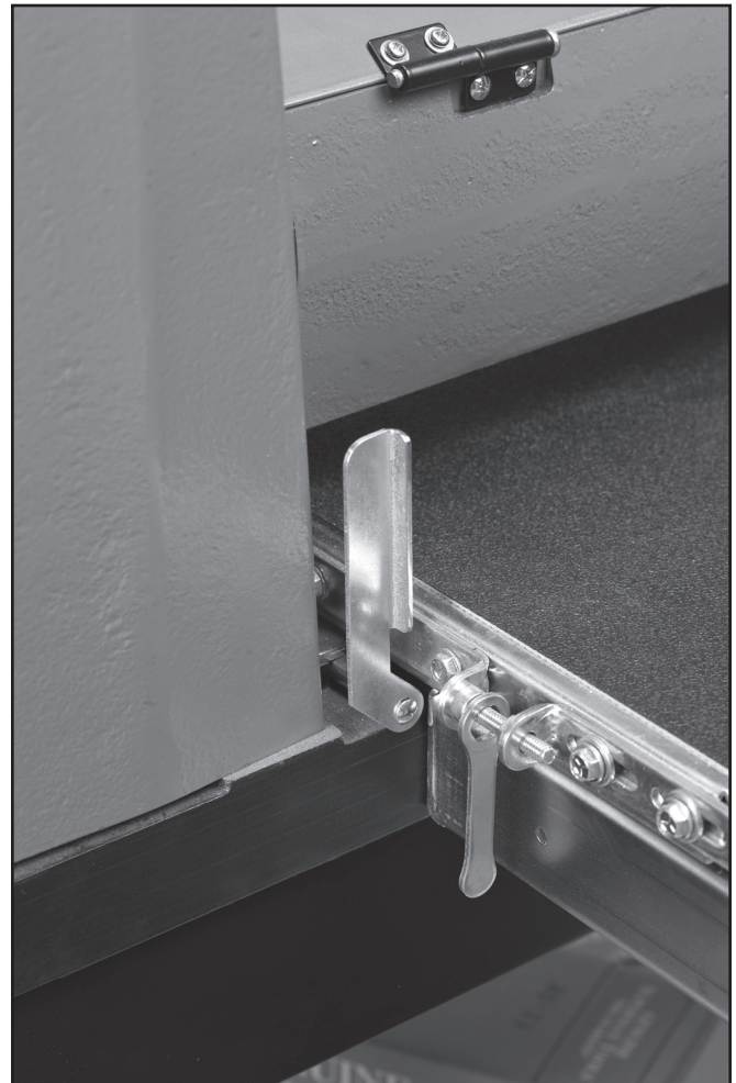
Fig. 9 Hanging wrench 1 of 2, for tracking conveyor
