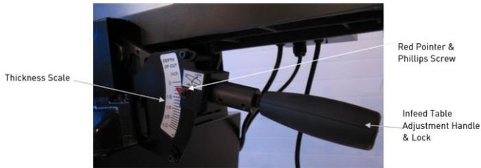
FIGURE 13: THICKNESS SCALE
