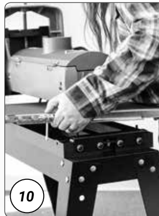
10 Open box 2 and remove conveyor from packaging and place on sanding unit. The conveyor motor should be nearest to the main motor and depth gauge.
