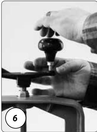
6 Install knob to height adjustment handle. First, finger tighten nut to knob. Thread stud from knob into hand wheel and tighten nut against hand wheel.
