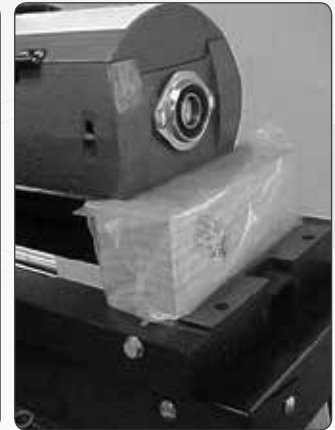
7 Turn the handle and raise sanding head to higher position to remove packing block from under carriage arm.
