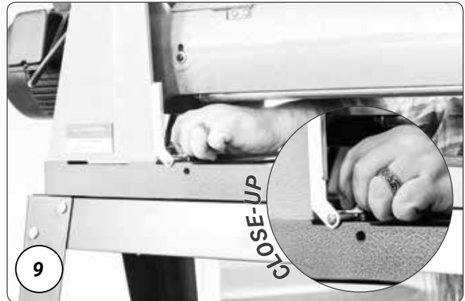
9 Next remove the 2 bolts on the inboard (right) side of the conveyor belt.
