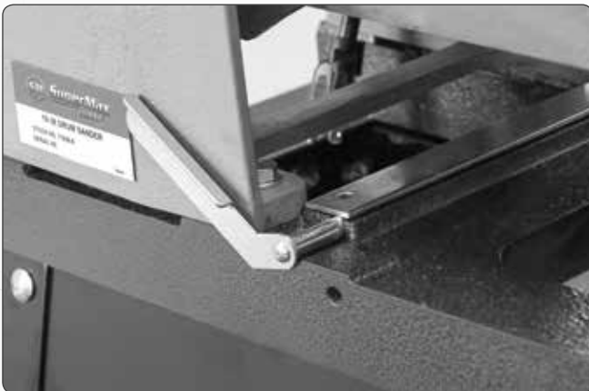
NOTE: Leave the silver plate, which is near the fast lever and under the motor, in place when removing bolts.
