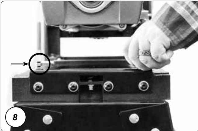
8 To prepare the unit for the installation of the conveyor belt, first remove the 2 bolts on the outboard (left) side of the conveyor belt.
