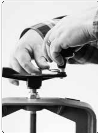
6 Install knob to height adjustment handle. First, finger tighten nut to knob. Thread stud from knob into hand wheel and tighten nut against hand wheel.
