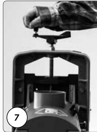
7 Turn the handle and raise sanding head to higher position to remove packing block from under carriage arm.
