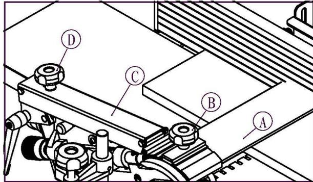
The height of the knife shaft cover (A) is carried out through the star screw (D). Turning to the right—the height of the cover plate is reduced. Turning to the left—the height of the cover plate increases.
