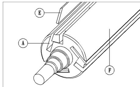
**The manufacturer recommends that the blade extends from 0.7 to 0.8mm**
