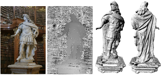
(a) One source view (b) Depth image (c) Front view (d) Back view Figure 4. The “Statue” dataset (consisting of 40 source views). The final mesh has 230460 triangles.
