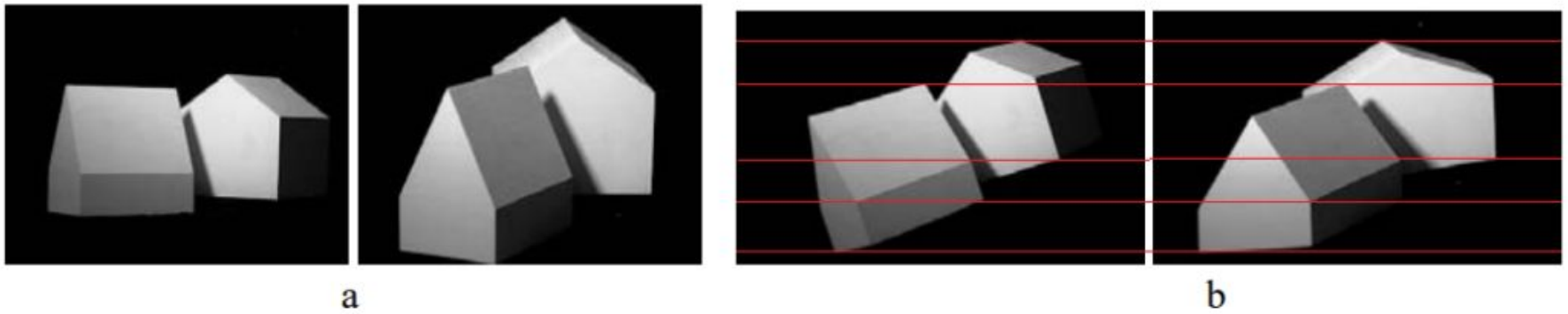
Fig. 11.11. Image rectification. (a) A pair of images of a house. (b) Resampled images computed from (a) using a projective transformation computed from F . Note, corresponding points in (b) match horizontally.
