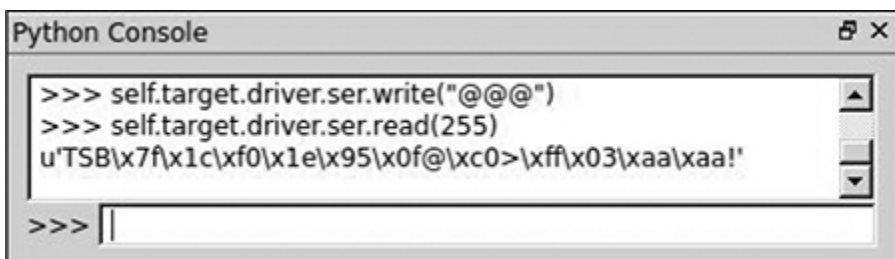
Figure 8-13: Sending @@@ via ChipWhisperer's Python console
