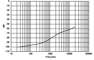
Figure 6.2 Typical Crosstalk vs. Frequency
