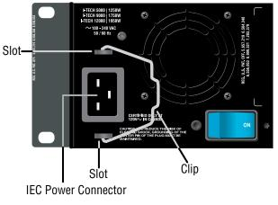
Figure 2.3 IEC Power Connector Clip
