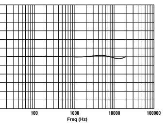
Figure 6.1 Typical Frequency Response (1W)
