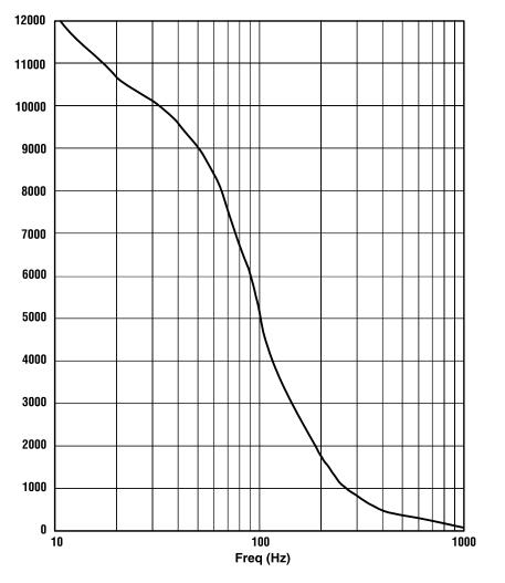
Figure 6.3 Typical Damping Factor vs. Frequency
