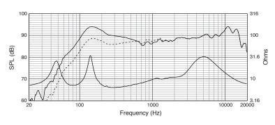
On-axis in half-space (2pi, solid line) and full-space (4pi, dotted line) at thru (8 $\Omega$ ) setting; input impedance (lower solid line)
