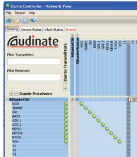
**Device Status** – Displays information about discovered Dante devices; double click a device name to enable its configuration.
