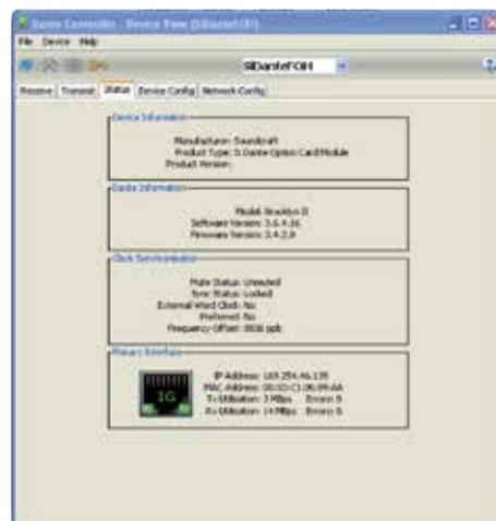
**Status:** The Status tab is used to view information about a Dante device, this information may be required for trouble shooting and checking software / firmware is up-to-date.
