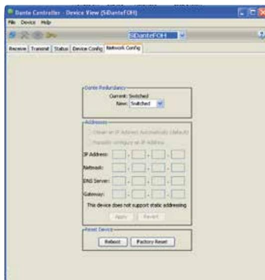
**Network Config:** This tab enables viewing and editing of Dante Redundancy mode.
