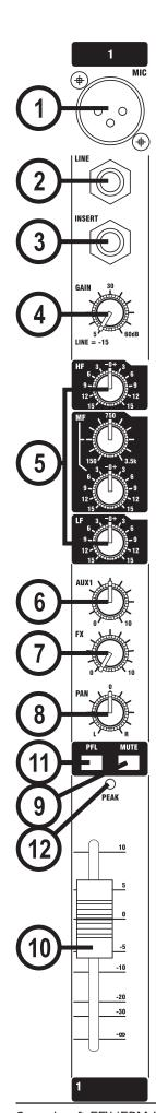
Note that some sound equipment, particularly that intended for domestic use, operates at a lower level (-10dBV) than professional equipment and will therefore need a higher gain setting to give the same output level. See "Initial Setup" on page 31 to learn how to set GAIN correctly.
