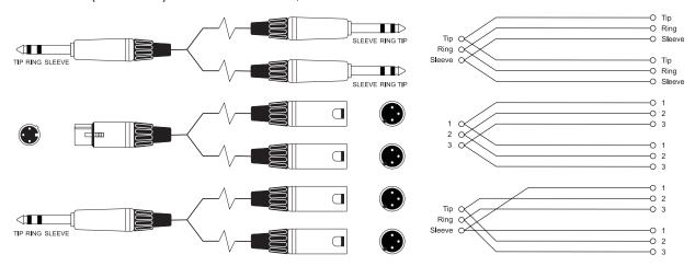
$\label{thm:local_phone_separator} \textbf{Note: for every doubling of headphones the load impedance is halved. Do not go below 150 Ohms.}$
