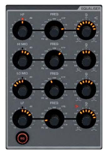
The channel EQ (Equaliser) section is used for sculpting the tonal (frequency-based) balance of the signal. The Impact EQ has four fully parametric, full range bands - LF and HF have switchable bell/shelf modes. You can check the EQ 'curve' via the Touch Screen Main Menu EQ button.
