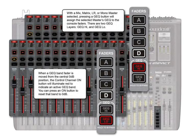
When any output channel is selected, the GEQ LO and GEQ HI buttons (FADERS button group) will assign 14 bands to the Control Channel Faders, colour-coded with red FaderGlow. Faders are centre (0dB position) detented with in use as GEQ bands.
