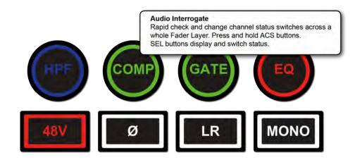
Audio Interrogate works for all status buttons on the Assignable Channel Strip:
