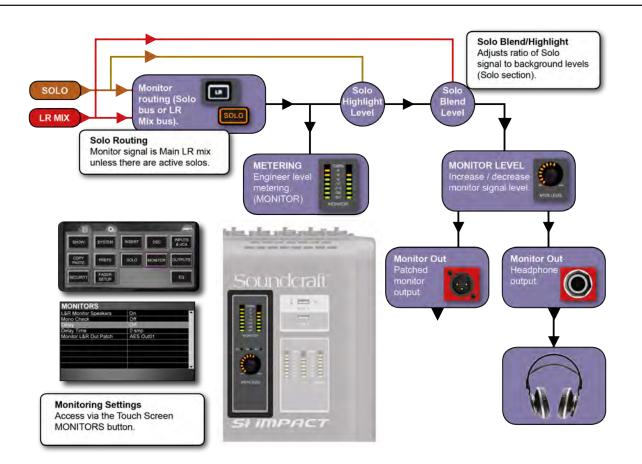
The active monitor signal is always available on the headphones output (located below the front of the console near fader 1). Monitoring level is normally controlled by the MON LEVEL encoder, though Main Fader and Mon Level Encoder functionality can be swapped using the LR/Mon Level Swap parameter in the Monitor Settings Menu. There is also a parallel Monitor Output Patch available allowing the engineer to connect control room speakers or headphone distribution, for example.
