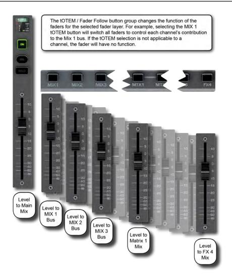
If your current fader layer is the default 'A' layer (all input channels), then pressing the MIX 1 tOTEM button will assign all channel faders to control the Mix 1 sends for those channels and the Mono control channel fader to control of the Mix 1 Master. This allows one-touch access to complete bus mixes.
