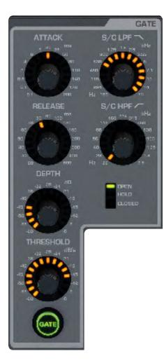
A Gate is a threshold-driven gain reduction process normally used to attenuate a signal when its level falls below the Threshold. Setting the Threshold just above a noise floor or background noise, for example, will allow the Gate to attenuate the source during periods when the main input (voice, instrument etc) is silent.
