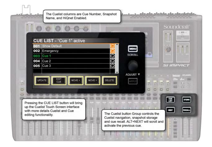
A snapshot is a 'picture' of the entire console state - all settings, patching, routing, and so on. A cue is essentially a snapshot of the console's state, plus a HiQnet Transmit (send a HiQnet venue preset event).
