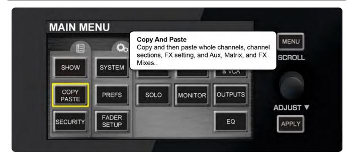
When you press COPY PASTE (Touch Screen Main Menu), or when you reselect a channel or bus while the COPY PASTE mode is active, the console's clipboard captures the state of that selection. If you have a channel selected, that channel's processing (except GAIN or 48V status') is copied; if you have a bus mix selected via the FADER FOL-LOW (tOTEM) buttons, that bus mix is copied.
