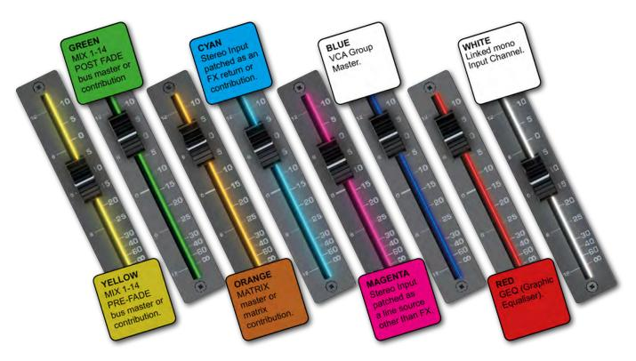
Several different functions can be assigned to the console faders, so it can be easy to lose track of which function is currently being controlled, especially when grabbing a fader in a hurry. The main principle of FaderGlow is to indicate the current fader function with colour, so more immediate recognition is possible. Soundcraft FaderGlow is fitted to all console faders that can change their function.
