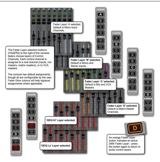
Each layer is made up of 24 Control Channels, plus the Left/Right and Mono/Centre main mix Control Channels.
