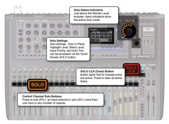
There are two main types of SOLO: PFL (Pre Fade Listen) and AFL (After Fade Listen). The difference between the two is the 'tap' where the solo source is taken from in the selected channel - pre- or post-fader. You can set whether Solos 'accumulate' (pressing a Solo button does not cancel other Solos) or 'Auto-Cancel' (pressing any solo cancels any other active solo) in the Solo Settings Menu.
