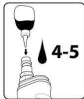
To lubricate the tool, apply air tool oils with ISO VG-32 viscosity and an automatic air line lubricator adjusted to supply 2 droplets per minute. If the use of an automatic air line is not possible, apply 4-5 droplets of air tool oil to the inlet pipe opening before each use of the tool. Using of oil with higher viscosity may deteriorate performance.
