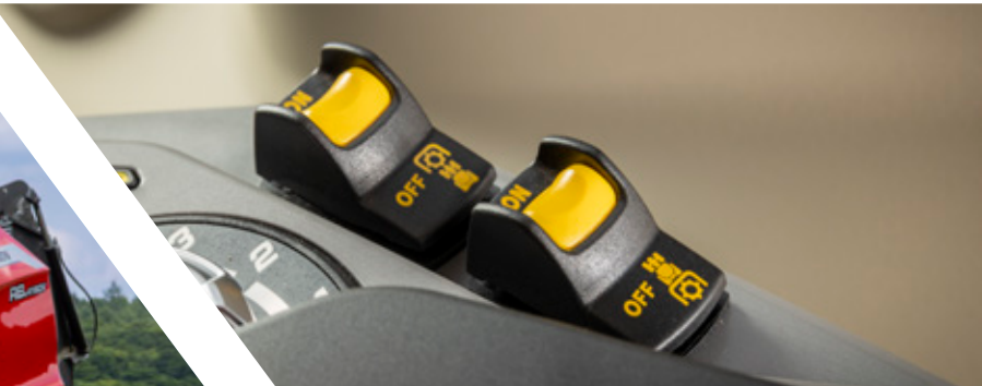
Electro-hydraulic PTO speed selection
