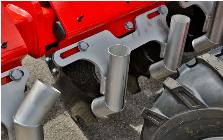
Stainless steel liquid manure outlets for long service life
