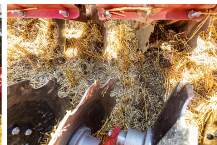
Paired arrangement of discs for maximum throughput
