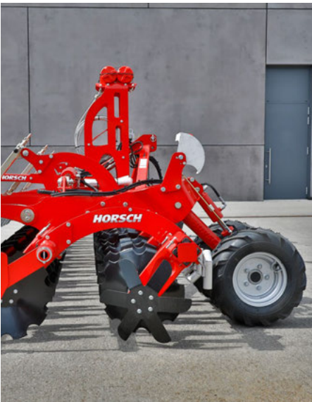
Liquid manure version without packer, with harrow to guarantee a low susceptibility to logging
