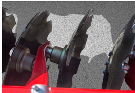
Disc serrated Ø 52 cm
