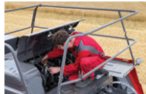
Knotter stack is easily accessible for servicing and maintenance.
