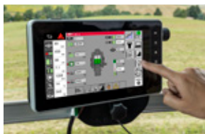
Standard Electronic Bale Length Control operates via the Fieldstar 5 baler terminal.
