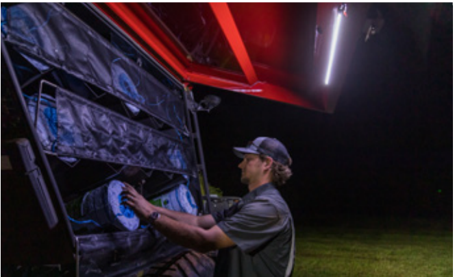
Dedicated twine box LED lighting helps refilling during the night.
