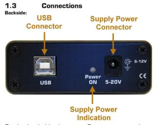
On the backside there are 2 connectors – the USB jack and the Power Supply jack. The device is supplied by a wall power supply unit which comes with the package. The external power supply is always necessary, even though USB is connected.
