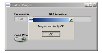
From now on, the hex-file is ready to be downloaded into PSØ81 on the target board. Of course you can download the hex-file into PSØ81 without the need to select the hex-file every time before the download. Once stored in the EEPROM of the production programmer you simply press the Start button and this triggers the download.
