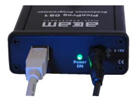
**Please note:** when plugging in the PicoProg Ø81 you need to make sure that it is power supplied by the external wall power supply unit (green LED on). The device is <u>not</u> supplied by USB!
