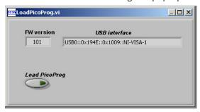
In the field *FW version* there should be a number displayed, e.g. 101, indicating the firmware version number. Also, in the *USB interface* field there should appear an USB descriptor like USB::Ox194E::Ox1009::NI-VISA-O. In the field *program cycles* you can define the number of possible downloads before the program is deleted automatically from the production programmer and no further downloads are feasible.
