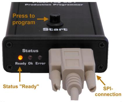
Make sure the PSØ81 on the target board has power supply also. Then press the **Start** button to initiate the programming of PSØ81. During the programming process the **Ready** LED is blinking. When the download is finished the result is indicated either by **Ok** or **Error**.
