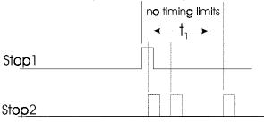
Give the triggersignal for the laser to the stop 1 input, the detector signal to the stop 2 input. In resolution adjust mode the first signal is interpretated as start. The order of signals in this set up is well defined, the start signal is identified. Time differences of 0s now can be measured. The loss in resolution, now only 250ps - can be compensated by sampling.
