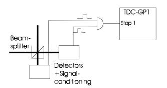
Using the resolution adjust mode the given stochastics allows high sampling rates and a reduction of the standard deviation down to the femtosecond range. The time difference itself must not have any noise, the GP1 itself delivers the necessary statistics of noise for the measurement.
