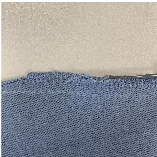
Overlock the seam allowances, keeping the underside of the dart facing up.
