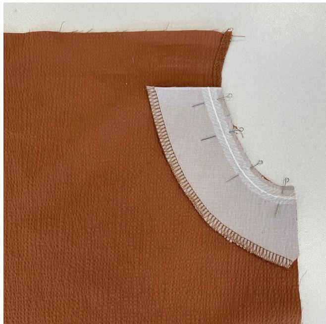
Place the top front and armscye facing pieces right sides together and align the edges. Pin and machine-stitch, backstitching at the beginning and end.
