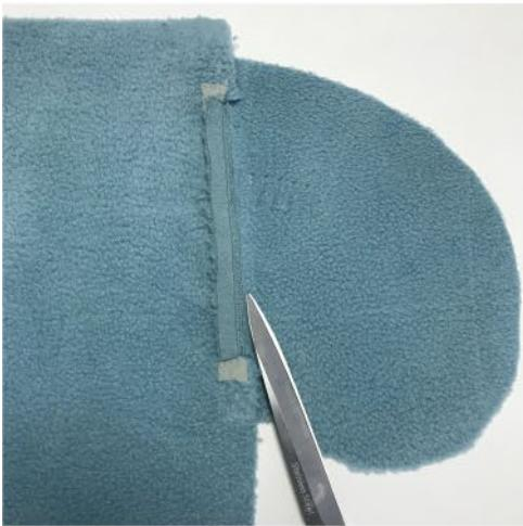
Trim the side seam allowance down to 2mm between the notches, as shown in the photo.
