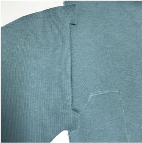
Working from the right side, understitch the pocket seam allowance to the pocket bag, 2mm away from the seam. Backstitch at both ends of the seam. Press.
